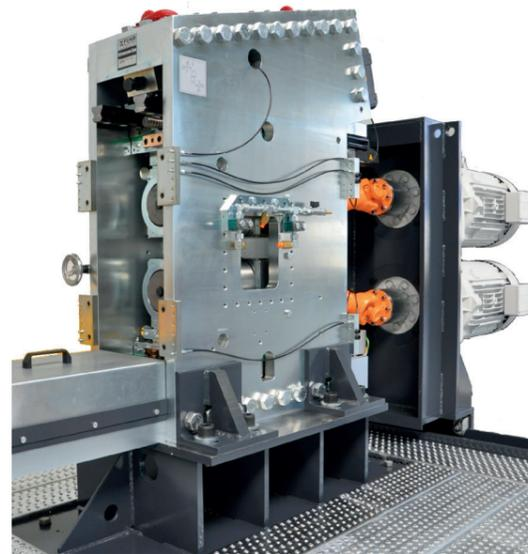
The 2-high rolling mills of the WSR type differ from the usual 2-high machines available for wire in their higher stiffness and the resultant higher precision of the flat wire produced.
